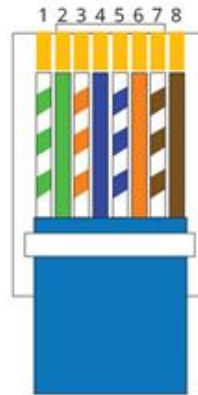
RJ45 Pinout T-568A
